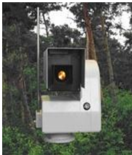
Figure 33. Automatic forest fire detector
